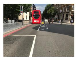
The right turn refuge island has been positioned to leave the eastbound lane approximately 3.0m wide. Emphasis should be given to the cycle route by placing pairs of Diag 1057 cycle logos centrally in the lane.
