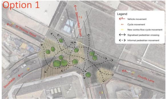
Fig 7: Full shared space with no priority given to vehicles in any direction. Drivers must negotiate various features (street trees etc) intended to create uncertainty and thereby reduce speeds.
