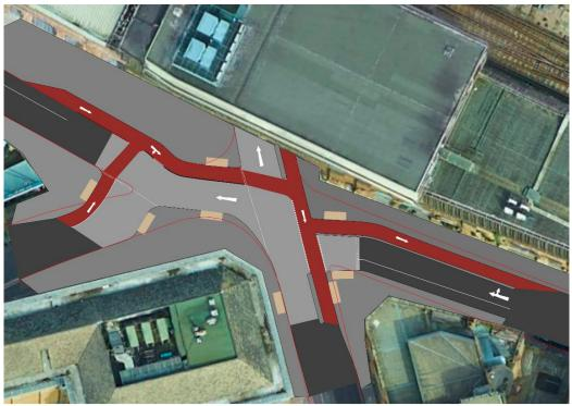
Fig 9: Major junction changes to introduce a priority junction with stagger and stepped contraflow cycle tracks. Incorporates significant kerb realignment and footway construction to shorten pedestrian crossing distances. Possible option to consider a zebra crossing on the St Thomas Street arm (not shown).
