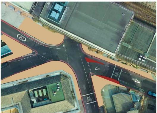
Fig 8: Simple junction changes introducing a slight stagger to emphasise priority and improve visibility of cycles travelling along Bermondsey Street. Minimal kerb adjustment / island construction.
